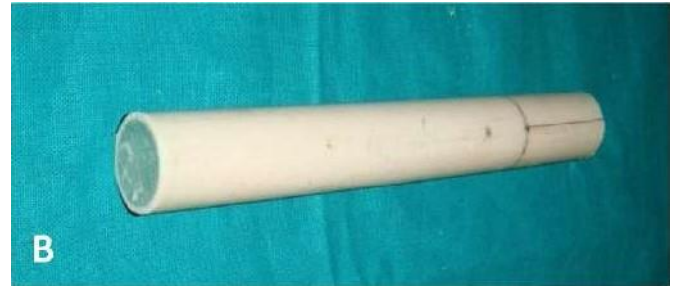
Fig. 2 B: Bottom opening of the PVC pipe blocked with dental stone
