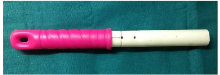
Fig. 7: Cap used over the Churro Fabricator to cover the projecting wires to ensure safety
