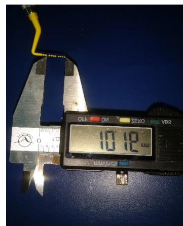
Fig 8: Measuring distance from tip of probe to the marking over probe with digital vernier caliper
